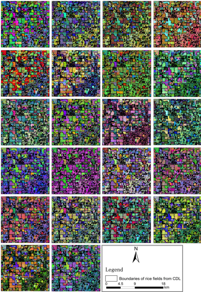
Fig. 14. Illustration of 64 deep temporal features extracted from raw time-series SAR images. Each image is composed of three temporal features in sequence as R/G/B-bands. The last image is composed of the 64th feature, the first feature, and the second feature. Polygons with black boundary denote rice fields from CDL.
