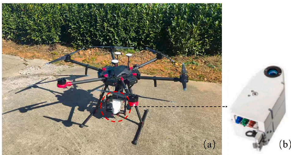
Fig. 2. UAV hyperspectral platform. (a) DJI M600 Pro UAV; (b) Rikola camera.
